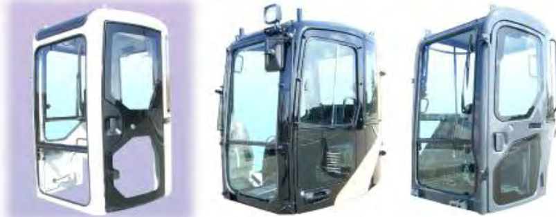
▼ Cabin for hydraulic excavator with small rear swing radius
